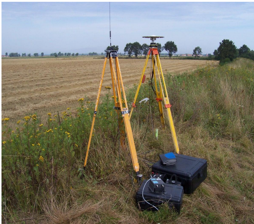
Fig. 2. Temporary RTK base station
