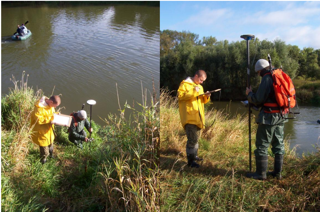
Fig. 5. RTK rover positioning near the river bank in open area
