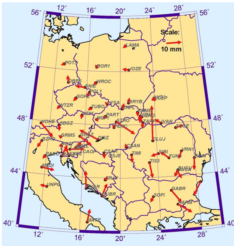
Fig. 3. Horizontal residuals from Helmert transformation between CEGRN 2003 and CEGRN 2005 coordinates.
