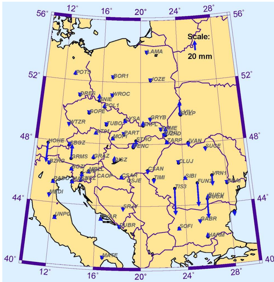
Fig. 4. Vertical residuals from Helmert transformation between CEGRN 2003 and CEGRN 2005 coordinates.
