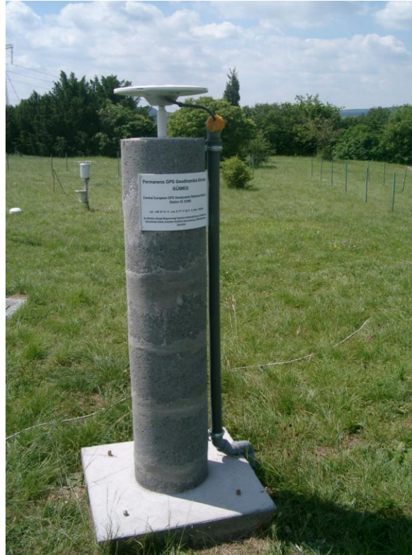
Fig. 3. The new Hungarian permanent CEGRN station SUME in Western Hungary
