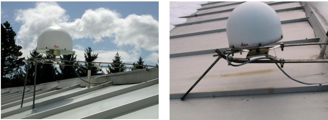
Figure 4. Antenna holder of ASIA originally (left) and after damage (right)
