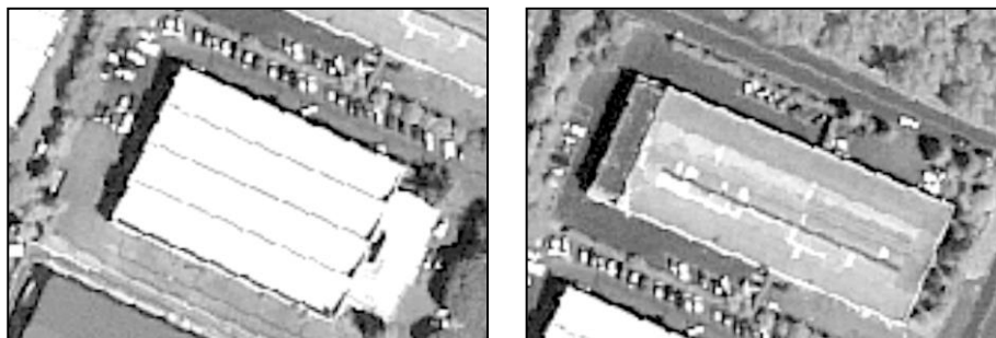
Fig. 3 Image enhancement: examples of root enhancement for eliminating shadows
