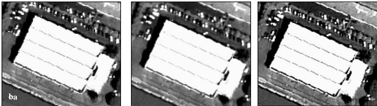
Fig. 2 Image enhancement: a. nearest neighbor resampling, b. bilinear interpolation, c. edge detection filter
