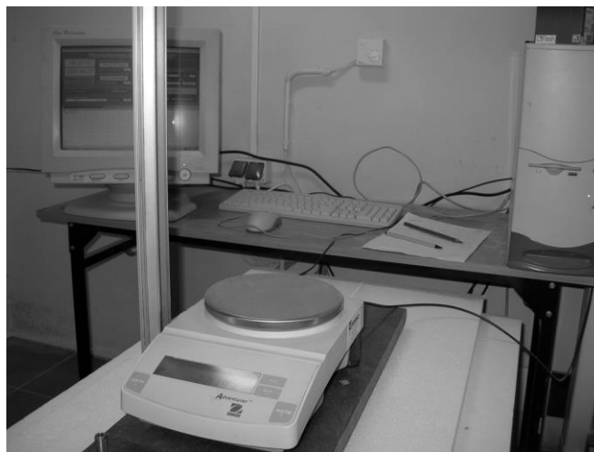
Fig. 1. The measuring system (the precise digital balance) with the controlling computer
