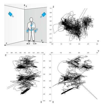
Fig. 1. Scheme of movement monitoring system (upper left) and projections of exemplary signal from single sensor on planes formed by pairs of axes
