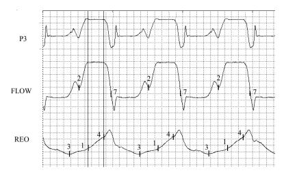
Fig. 8. The method for determination of characteristics points on the bioimpedance signal.
