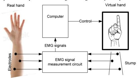
Fig. 6. The block diagram of the measurement system for identifying the relation between the hand movement and EMG signal taken from the muscles of forearm and stump.
