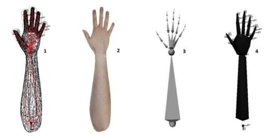
Fig. 4. Tiering in the engine. 1) location of component layers in the limb (2, 3 and 4), 2) graphical model, 3) bones of graphical model, 4) physical model.
