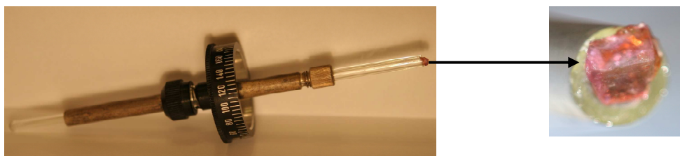
Fig. 6. A ruby crystal – the secondary reference during the measurements of free radicals concentration.
