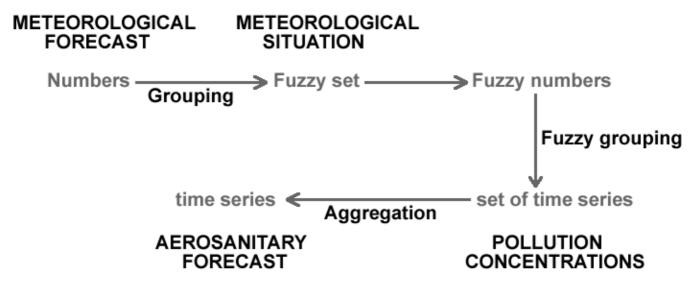
Fig. 1. The stages of Air Pollution Forecast Model.
