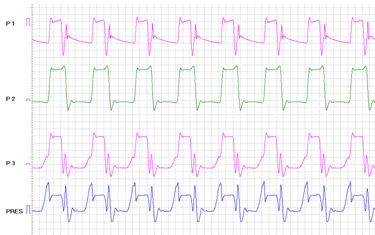
Fig. 7. Pressure waveforms recorded at various locations of the VAD during the experiment with the hybrid flow model (P1 – separated transducer – pressure in the outflow connector; P2 – reference NPC-100 transducer – control side; P3 – reference NPC-100 transducer – pressure inside the blood part of the VAD; PRES – reference NXPG-2 transducer – pressure in the inflow connector).
