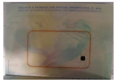
Fig. 2. In UK passports the chip and antenna are directly visible.
