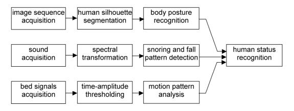
Fig. 2 Block diagram of the residential behavior tracking system [12].
