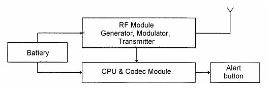
Fig. 2. Block diagram of an emergency radio transmitter
