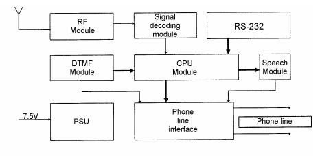
Fig. 3. Block diagram of an automatic telephone notifier
