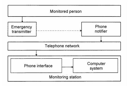
Fig. 1. System components
