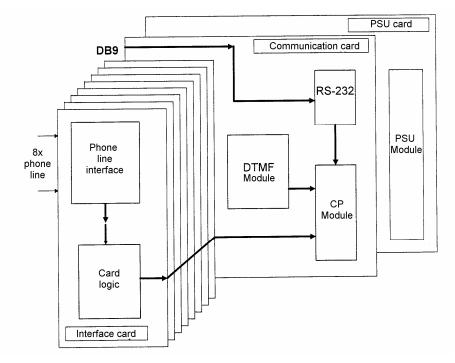
Fig. 4. Telephone line interface system
