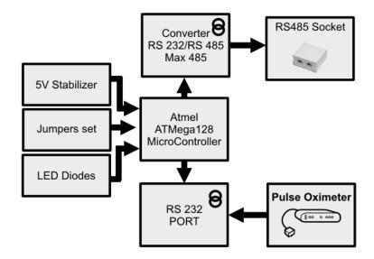
Fig. 2. Hardware structure of interface unit
