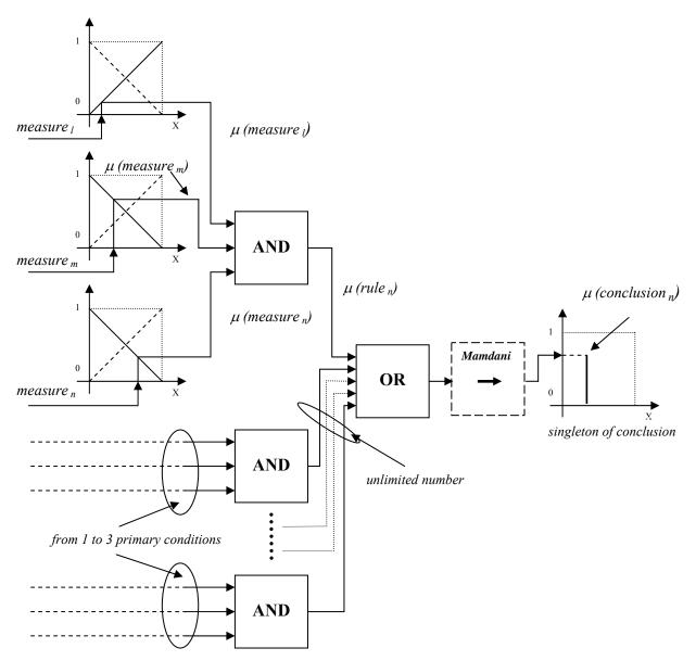
Fig.2. The fuzzy inferring flowchart
