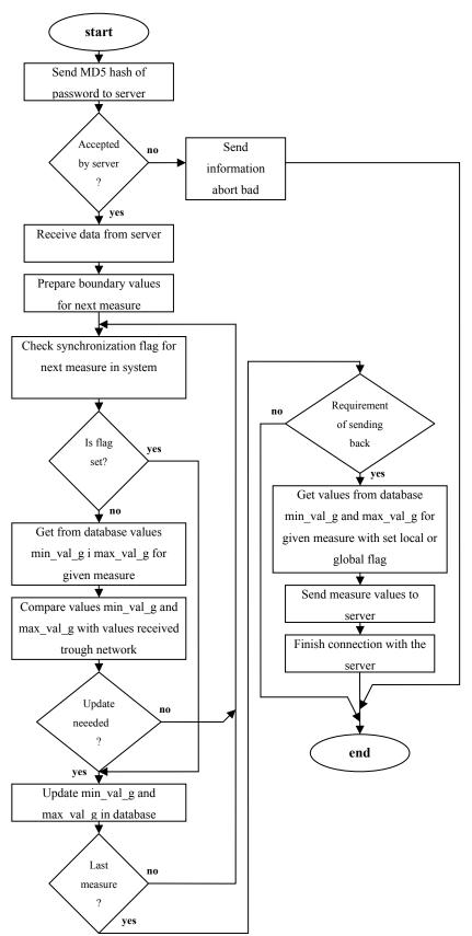
Fig.7. Synchronisation processes flowchart of pattern data finding
