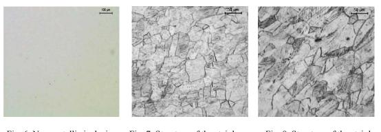
Fig. 6. Non-metallic inclusion stainless steel, longitudinal microsection magn. x100
