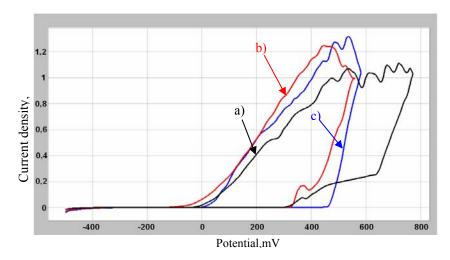
Fig. 14. The anodic polarization curve for plates used for 25 month: a) end side 1, b) middle side, c) end side 2
