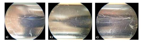
Fig. 9. Plate with the surface damage (24 month): a) end side 1, b) middle, c) end side 2
