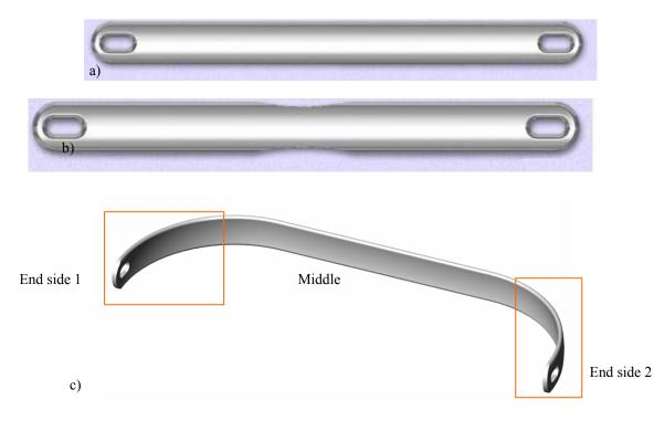
Fig. 2. Fixation plates: in initial state - a) narrow, b) wide [20], - c) after bending
