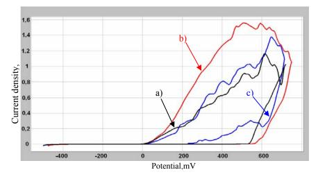
Fig. 15. The anodic polarization curve for plates used for 25 month: a) end side 1, b) middle side, c) end side 2
