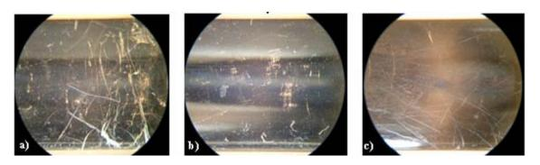
Fig. 10. Plate with the surface damage (25month): a) end side 1, b) middle, c) end side 2
