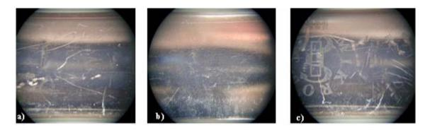
Fig. 11. Plate with the surface damage (26 month): a) end side 1, b) middle, c) end side 2
