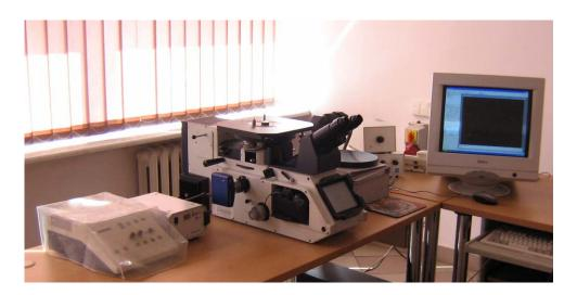
Fig. 5. The MEFCA (LEICA) light microscope
