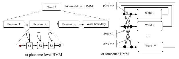
Fig. 1. The structure of HMM used in the isolated utterance recognition
