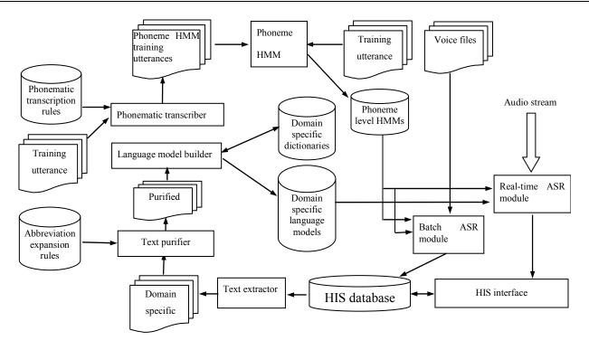
Fig. 2. The architecture of ASR module focused on integration with hospital information system
