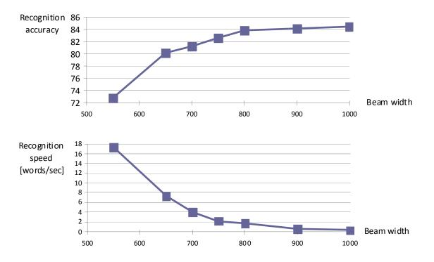
Fig. 4. ASR time and accuracy as a function of beam width
