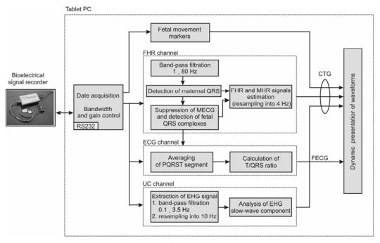
Fig.1 Structure of the remote instrumentation for the acquisition and analysis of the fetal ECG and EHG signals.
