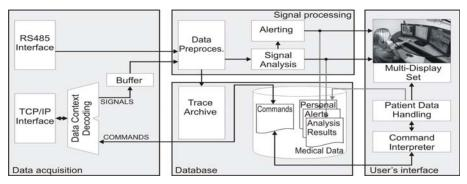
Fig.4 The structure and interactions between different components of the Surveillance Centre from the fetal monitoring system. 94
