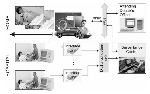
Fig.2 A structure of centralized fetal monitoring system incorporating remote devices as well as classic bedside monitors located in hospital.
