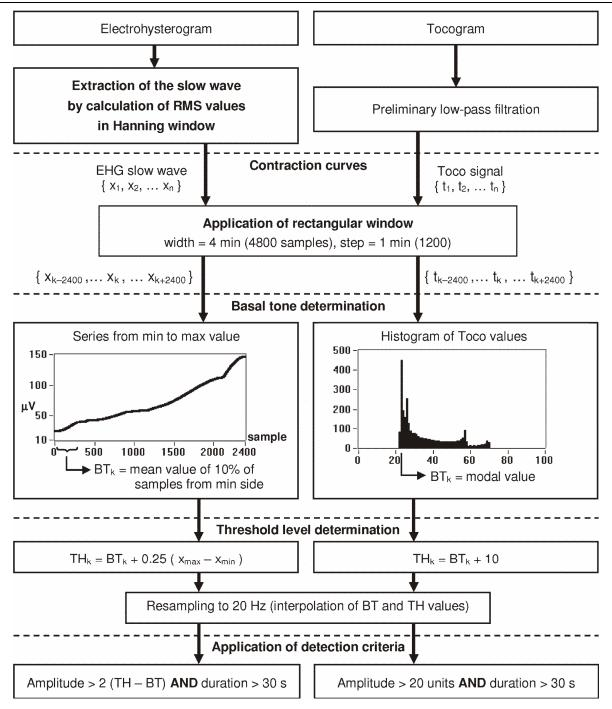
Fig.3. Overview of the algorithms for uterine contractions detection in the electrohysterogram and tocogram.
