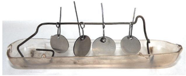
Fig. 1. Samples prepared for the corrosion resistance tests of the valve steel in diesel exhaust gas on a hanger in a glass bowl
