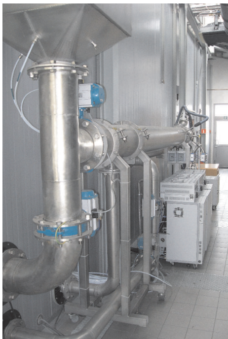
Fig. 9. Two views of the dilution tunnel (facing downstream), showing the heated OVN units for measuring emissions of THC, CH 4 and NO x positioned under the tunnel
