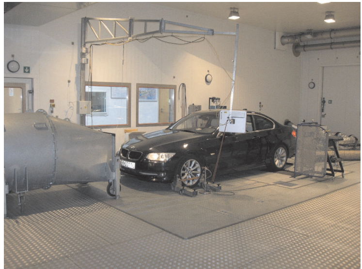
Fig. 3. Internal view of the climatic chamber, showing the windspeed fan and driver's aid mounted in front of a vehicle positioned on the chassis dynamometer
