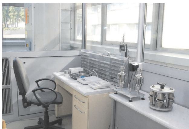
Fig. 12. The balance, filter conditioning racks and filter cartridges in the climate controlled weighing chamber
