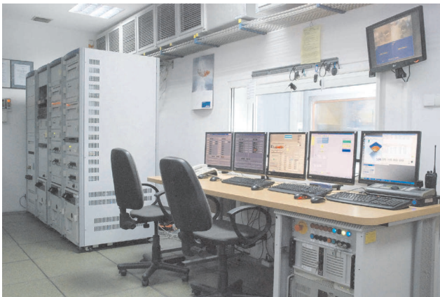
Fig. 6. View of the operator's workstation in the upgraded laboratory, showing the analyser racks (left), including the recently added MEXA7500DEGR bench; and the monitors of the computer control systems (left to right: raw emissions, bag and diluted emissions, VETS control system, chassis dynamometer control system, climatic chamber control system; above: chamber CCTV monitor)
