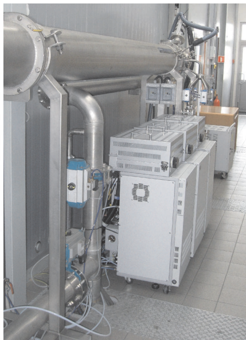
Fig. 9. Two views of the dilution tunnel (facing downstream), showing the heated OVN units for measuring emissions of THC, CH 4 and NO x positioned under the tunnel
