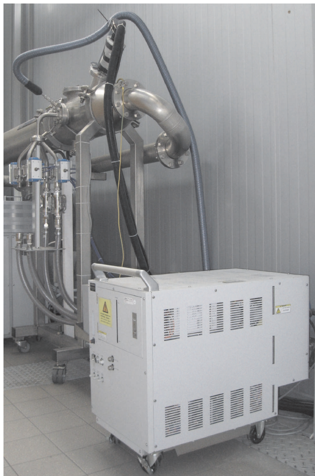
Fig. 11. Dilution tunnel (looking upstream), showing the filter cartridge installation (left), the heated particulate number counter sample transfer tube (blue), the heated HFID transfer tube (black), and the HORIBA 2000-SPCS PN counter (foreground)
