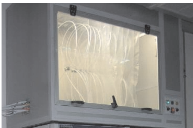
Fig. 8. Sample bags within their climate-controlled enclosure
