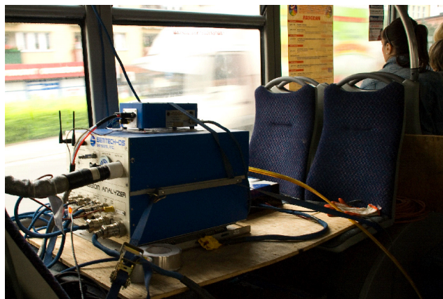
Fig. 4. Research apparatus used in the study exhaust emission buses in real traffic conditions in Rzeszow
