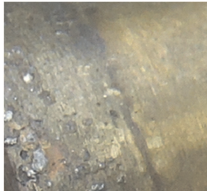
Fig. 10. Damaged transverse bearing: a) scale 1:1, b) scale 10:1
