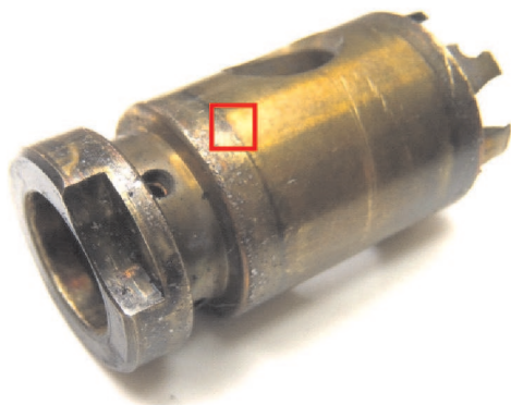
Fig. 10. Damaged transverse bearing: a) scale 1:1, b) scale 10:1
