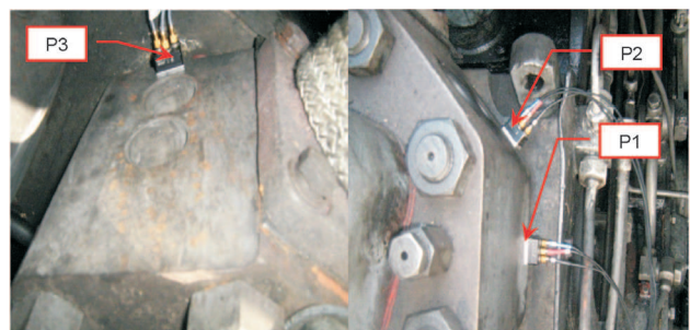
Fig. 2. Distribution of acceleration transducers on the cylinder head, engine a8C22
