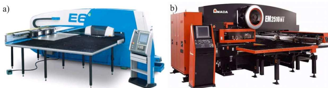
Rys. 8. Wykrawarki rewolwerowe: E6 firmy Finn Power (a) i EM 2510NT firmy Amada (b) [9] Fig. 8. Turret punch presses: Finn Power E6 (a) and Amada EM 2510NT (b) [9]
