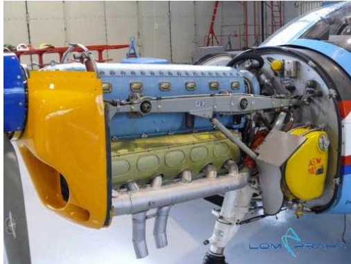
Fig. 2. The engine - Avia M 337 AK supercharged (M 337 C) [10]
