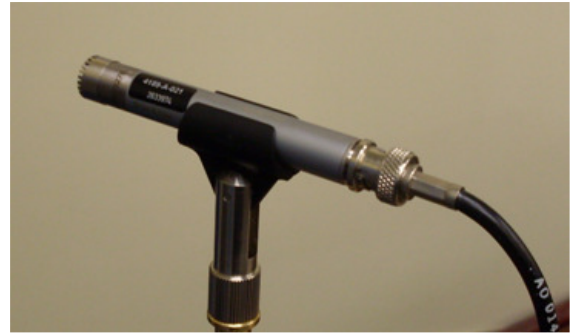
Fig. 4. Microphone ½" Typ 4189 by Brüel & Kjær
