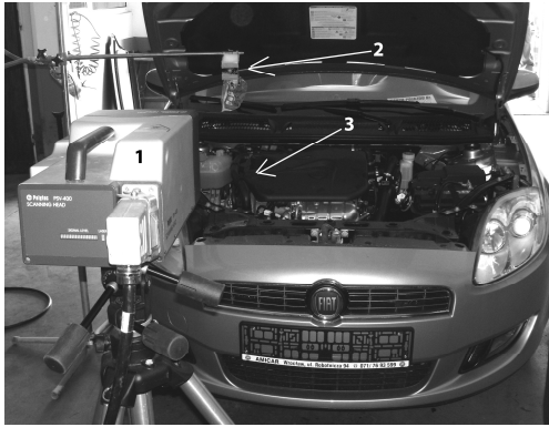
Fig. 3. Test rig: 1- laser probe, 2- mirror, 3- place of laser beam reflection
