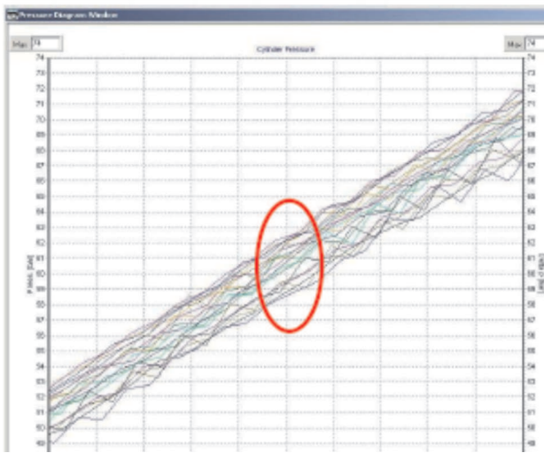
Fig. 19. Compare pressure at 15° CA before TDC
