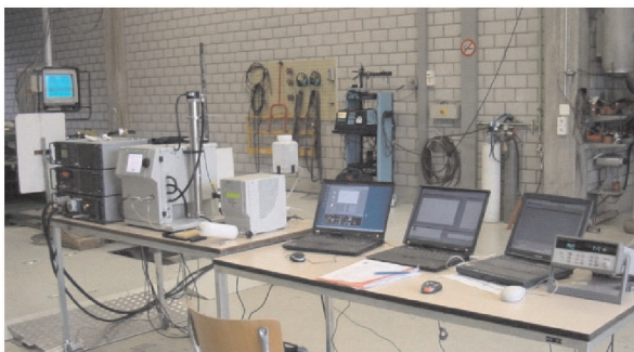
Fig. 3. Sampling and measuring set-up for nanoparticulate analysis of scooters
