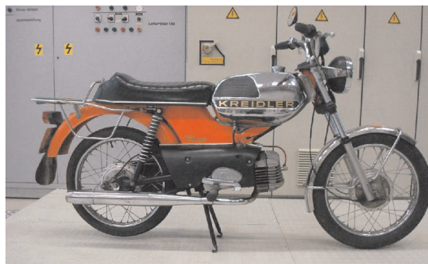
Fig. 1. Investigated 2-S Scooter: a) Piaggio Typhoon 2-S 50 cc, b) Kreidler Florett 2-S 50cc
