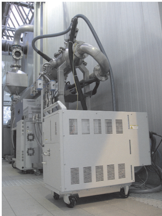
Fig. 11. Dilution tunnel (looking upstream), particulate number counter sample transfer tube (blue), HFID transfer tube (black), and HORIBA 2000-SPCS PN counter (foreground)
