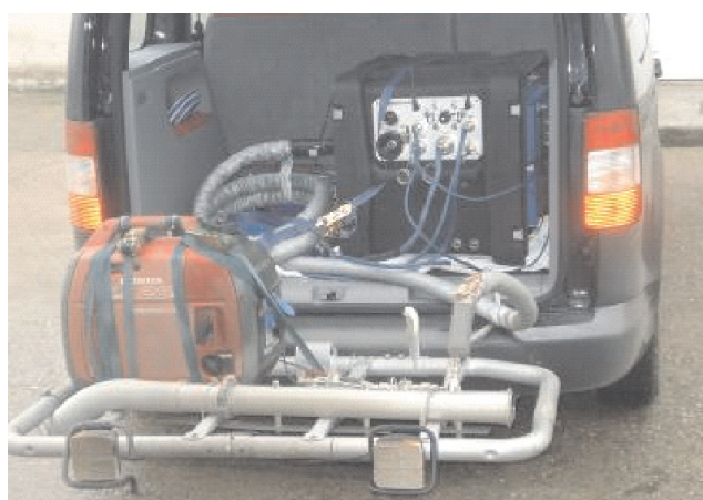
Fig. 7. The view of SEMTECH DS analyzer mounted in the vehicle during the tests
