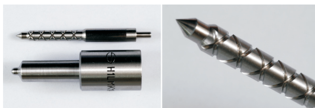
Fig. 2. Atomizer of a 359 engine with preliminary fuel treatment system and turbulizing channels
