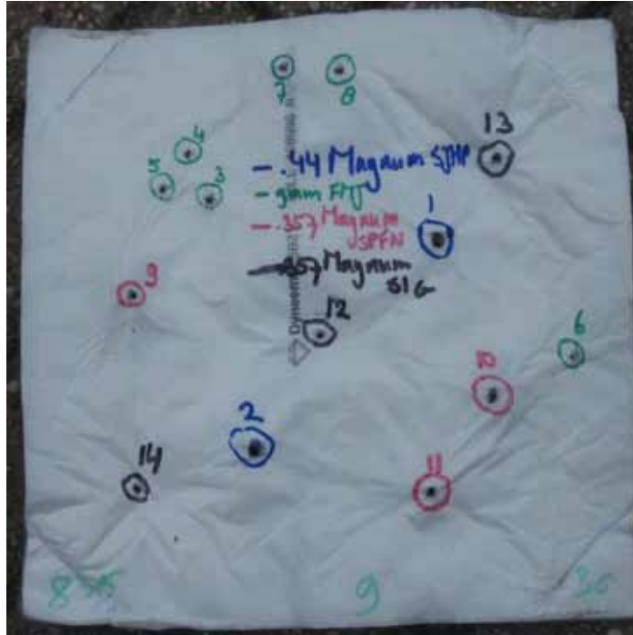
Figure 2: A package of Dyneema® SB21 with multiple impacts from various bullets, including close to the edge and close to other impacts
