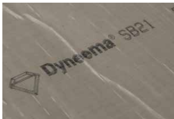
Figure 1: Print on Dyneema® UD with type and batch number
