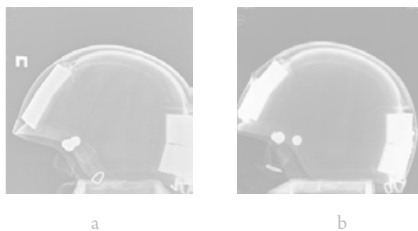
Figure 1. X-ray photographs of increased protection level helmet with strengthened frontal and rear areas: a - before submachine-gun fire; b - after the fire.
