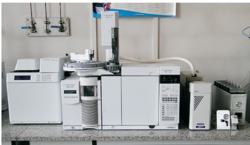
Fig. 3. Chromatography system: GC Agilent 7890A with autosampler 7683B, splitter and FID detector, MSD Agilent 5975C mass selective detector, Agilent G1888 headspace sampler, Markes UNITY2 thermodesorber and Markes \mu -CTE (Micro-Chamber Thermal Extractor), situated within BOSMAL's chemical laboratory
