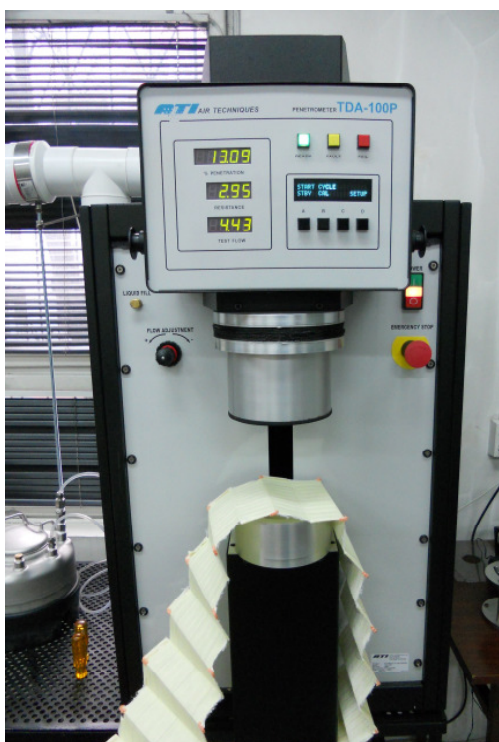
Rys. 3. Tester TDA – 100P firmy ATI AIR TECHNIQUES [3]
