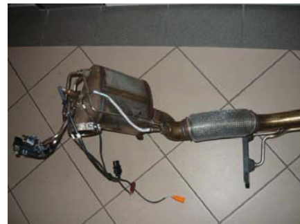
Fig. 14. View of the DPF fitted in Skoda exhaust aftertreatment system
