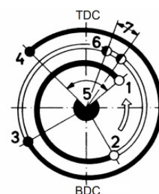
Fig. 2. Static fuel injection valve and valve gear timing diagrams of the MB820 type diesel engine
