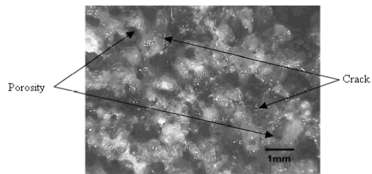
Fig. 1. Typical optical surface morphology of the OPC surface glaze generated with the CO 2 laser (Lawrence, 2004).
