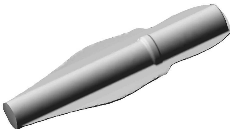
Fig. 3. Numerically generated model of a forging with a flash
