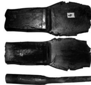
Fig. 3. Sample of the NiCrN ingot after free swelling in flat dice
