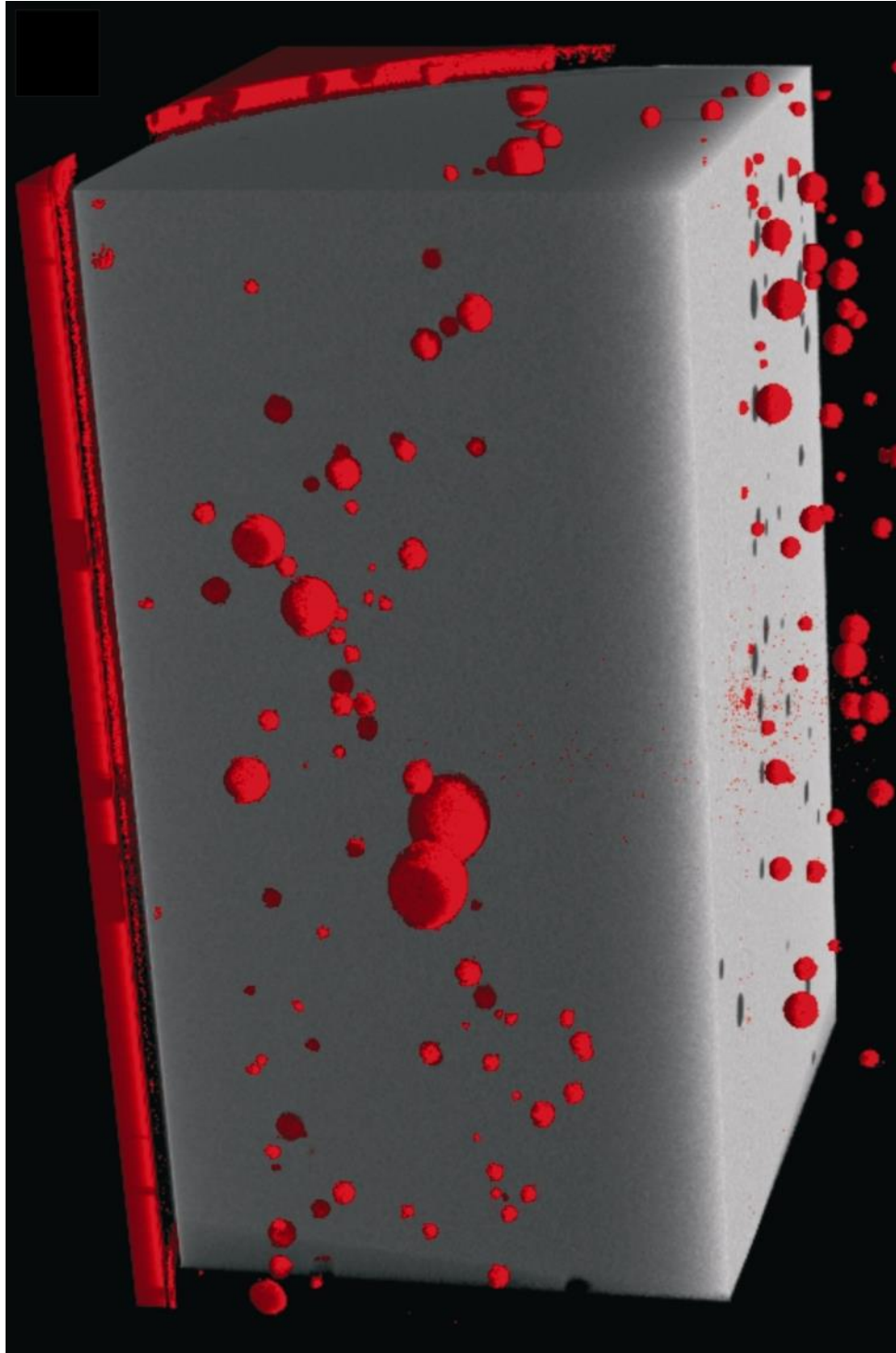
Fig.1 Image generated through CT scanning of a vertical core through bubbly gel (described in reference [3]), used for validation purposes during the construction of the device described in this paper. In the image, the host gel near the edges of the quadrant has been clipped back to show the presence of the bubbles. For scale, the largest bubble visible has a diameter of \sim 1\text{mm}
