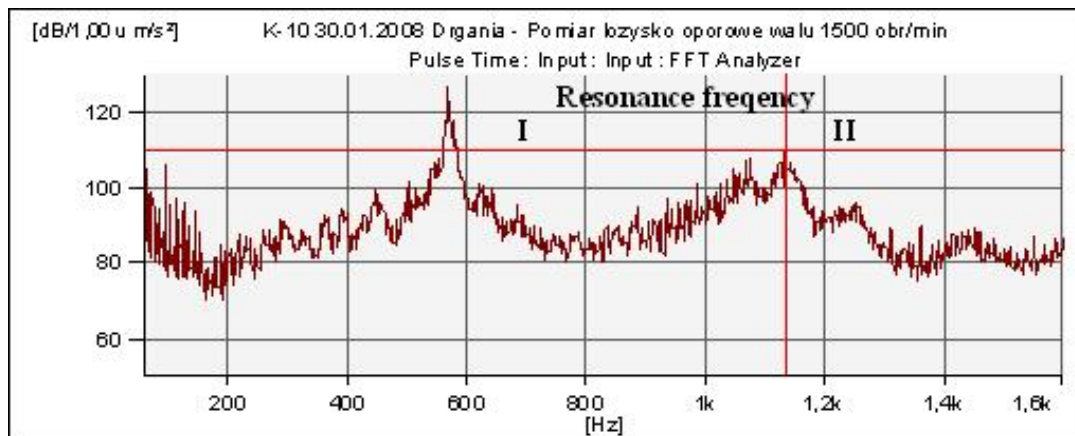
Fig.6 Spectrum of accelerations recorded in the shaft's thrust bearing; n = 1500 rpm
