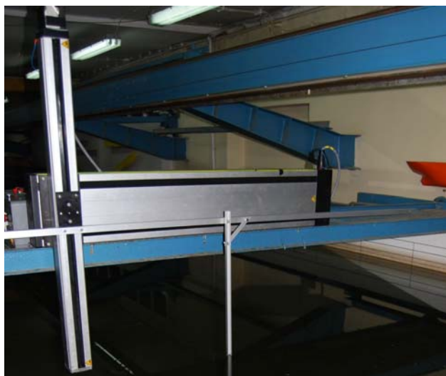
Fig.11. Precision arm with a hydrophone to directivity characteristic measuring
