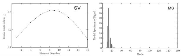
Next, we show analogous figures for the first iteration under the criterion of the maximum SNR gain as was formulated in Sec. III. In this case, the eigenvalues and eigenvectors are calculated directly from Eq. (15). The adaptive corrections of the source vector (SV) and the excited modal spectrum (MS) are demonstrated here to illustrate how the algorithm of the signal wavefield control works.
