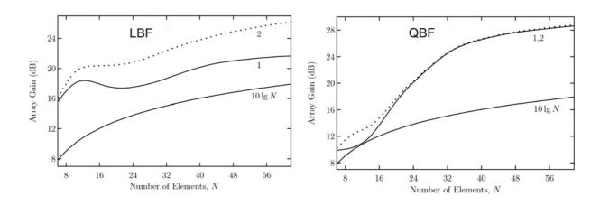
We also emphasize that the second and subsequent iterations almost does not lead to any enhancement of the gain. For example, for the full-size array the LBF gain values versus the number of the adaptive iterations are the following: G(0) = 21.7 dB, G(1) = 28.5 dB, and G(2) = 28.6 dB. This means that the adaptive algorithm presented is rather effective and provides the fast convergence to the optimal (for the given set of parameters) array gain performance.
