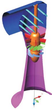
Figure 1. Schematic view of the flow system of investigated model turbine.
