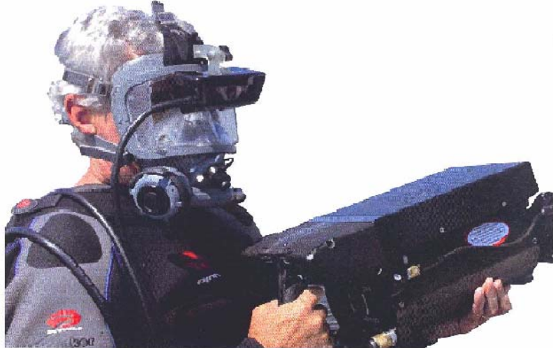
Fig.5 A diver with a camera and glasses type display. (Courtesy of DIDSON DH)
